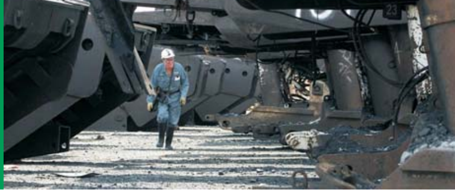
Left: Ian McDonald, Crew Leader, inspecting longwall hydraulic chocks removed from underground.
